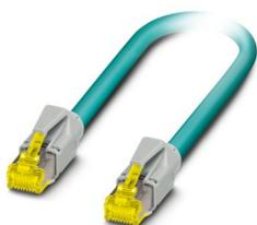
Patch cable, CAT6<sub>A</sub>, 4-pair, shielded, connection not crossed (line), assembled at both ends with RJ45/IP20 connectors, outer sheath material: PUR, length: 2.0 m
