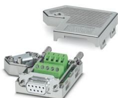
D-SUB connector, 9-pos. socket, one 35° cable outlet, universal type for all systems, pin assignment: 1, 2, 3, 4, 5, 6, 7, 8, 9 to screw connection terminal block
