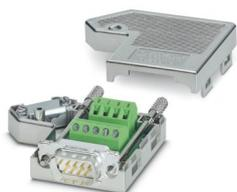
D-SUB connector, 9-pos., pin, one 35° cable outlet, universal type for all systems, pin assignment: 1, 2, 3, 4, 5, 6, 7, 8, 9 to screw connection terminal block
