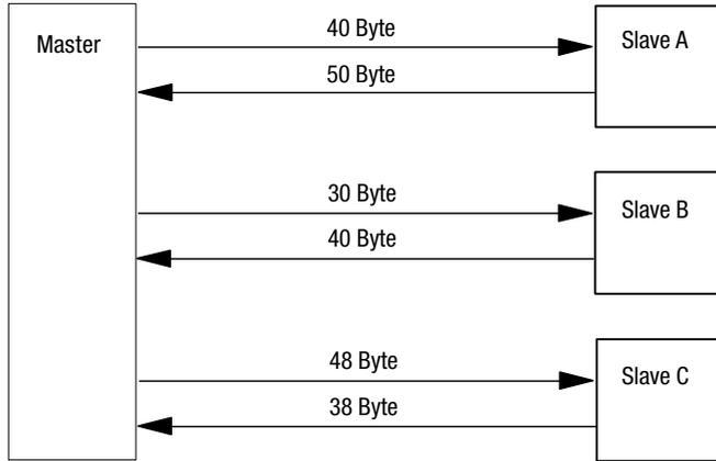
Figure 26: Data exchange between master and slaves
