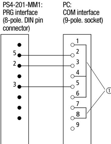
Figure 7: Pin assignment of the ZB4-303-KB1 programming cable
