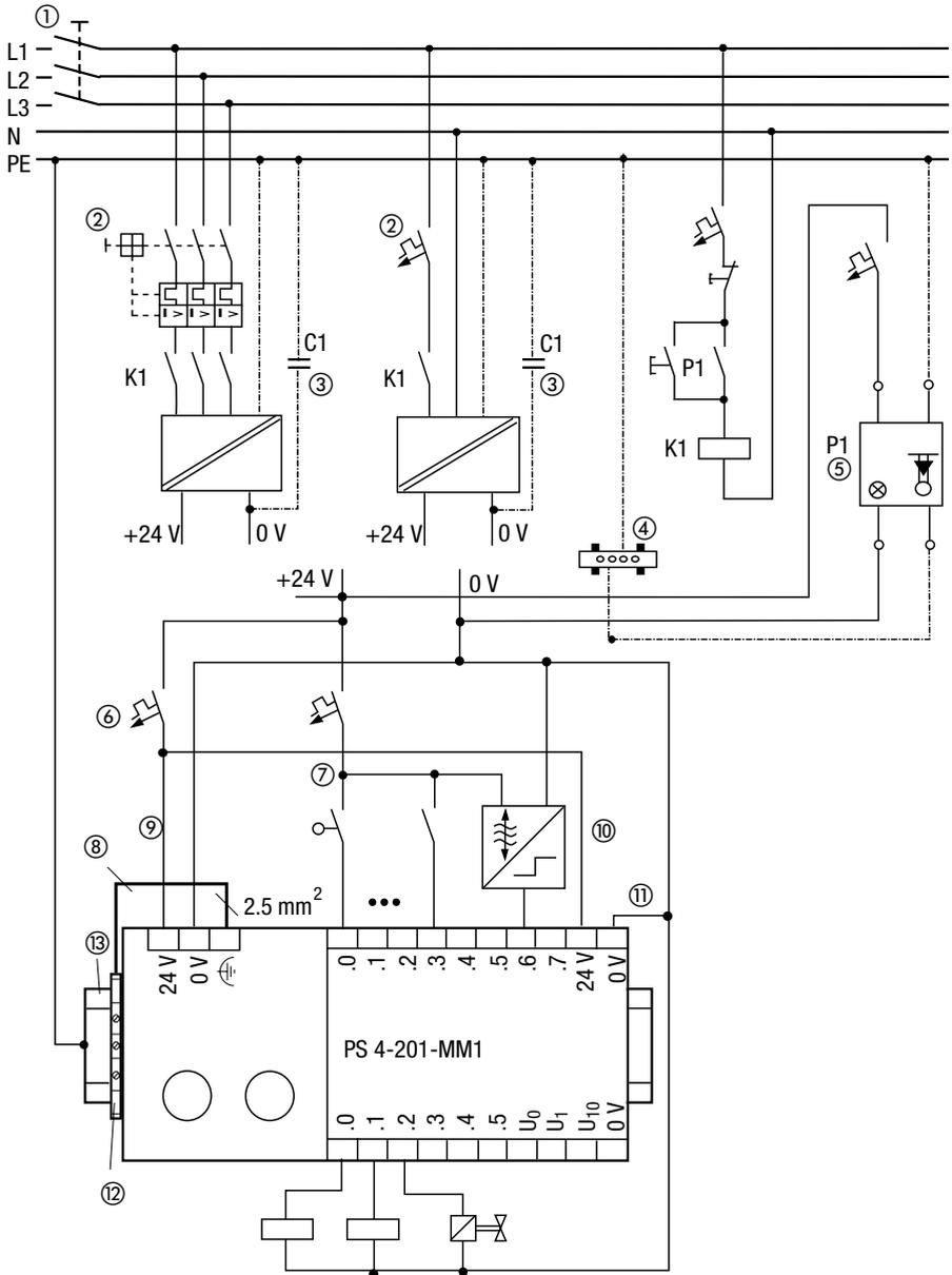
Figure 12: Common power supply wired for non-grounded operation
