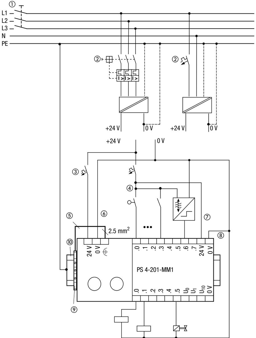
Figure 11: Common power supply wired for grounded operation
