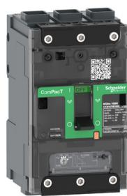
circuit breaker ComPacT NSXm B (25 kA at 415 VAC), 3P 3d, 125 A rating TMD trip unit, EverLink connectors
